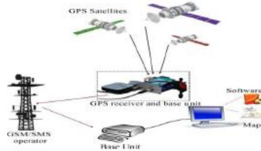
Fig. 6. Block diagram of GPS tracking system.
