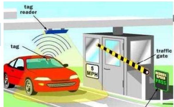
Fig. General diagram of RFID based Toll Collection System
