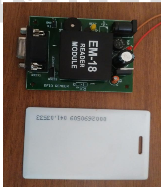
Fig. 3 RFID reader and Tag
