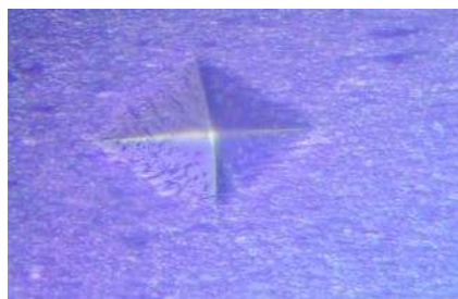
Fig 9. Micro Hardness Indentation of AA6061 And AA6082
