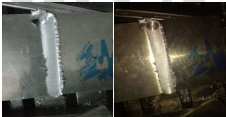
Fig 4. Weldments of AA6061 and AA6082
