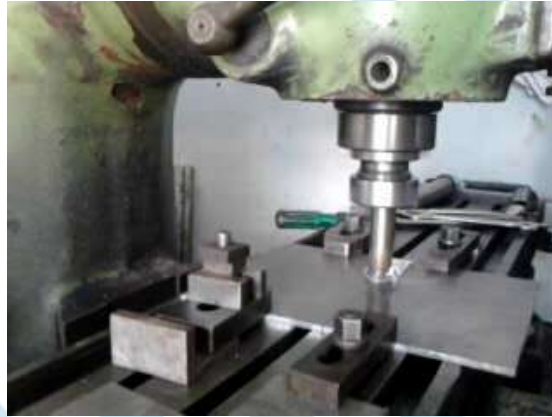
Fig 3. Friction stir welding Experimental Setup
