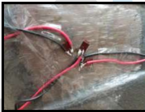
Figure 7:- strain gauges on the product
