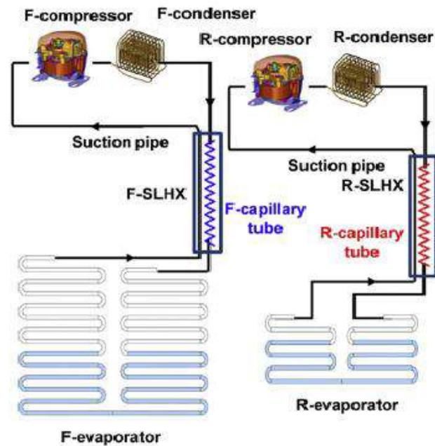
Fig 2.11 schematic diagram of a the dual-loop cycle <sup>[12]</sup>
