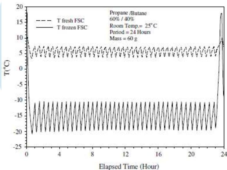
Fig 2.3 Temperature profiles during 24 h in the fresh food storage compartment and in the frozen food storage compartment <sup>[4]</sup>
