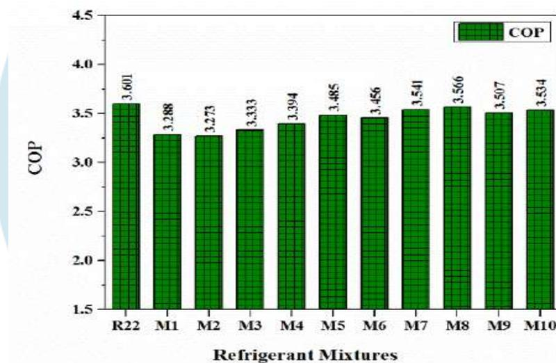
Fig 2.5 COP of various refrigerant mixtures <sup>[4]</sup>
