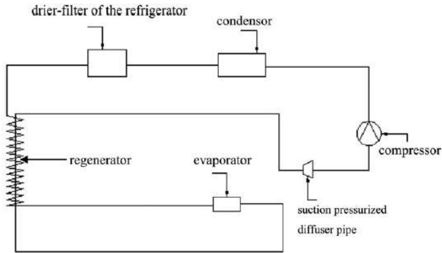
Fig 2.8 Refrigeration system with suction-pressurized and energy-saving diffuser pipe <sup>[10]</sup>
