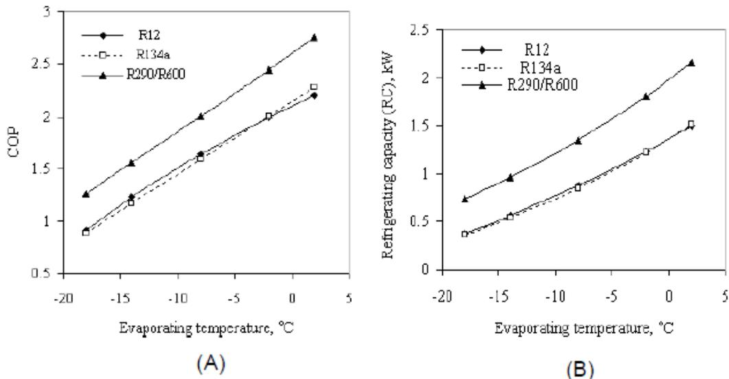
Fig 2.12 (A) Effect of condensing temperature on COP (B) Effect of condensing temperature on RC <sup>[14]</sup>
