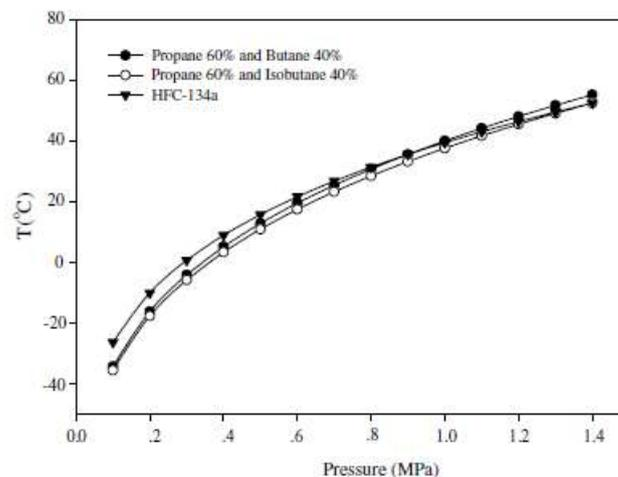
Fig 2.4 Comparison of saturated pressure and temperature for various refrigerants <sup>[4]</sup>
