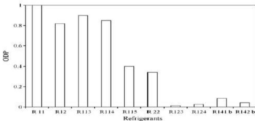
Fig 2.1 Ozone depletion potential of pure CFC and HCFC refrigerants <sup>[2]</sup>
