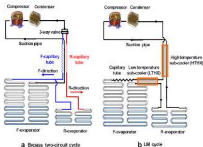
Fig 2. 10 (a) bypass two circuit cycle (b) LM cycle <sup>[11]</sup>
