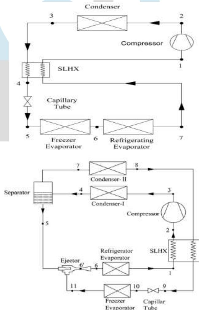
Fig 2.13 (A) Schematic diagram for the TVRC cycle (B) Schematic diagram for the MVRC cycle <sup>[15]</sup>
