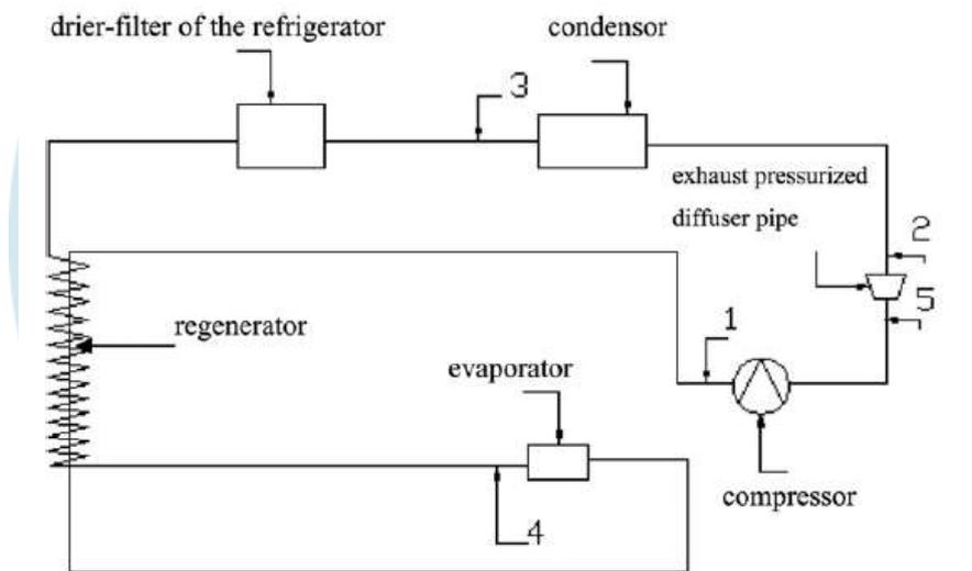
Fig 2.9 Refrigeration system with exhaust-pressurized and energy-saving diffuser pipe <sup>[10]</sup>
