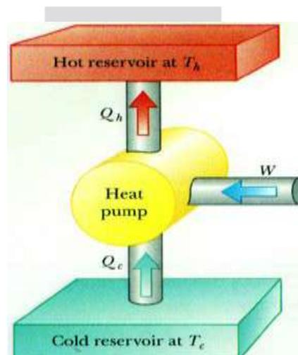
Fig1.1 Reversed Heat Engine<sup>[1]</sup>
