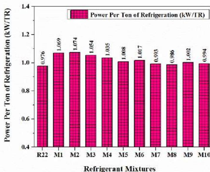
Fig 2.6 Power per ton of refrigeration for various refrigerant mixtures <sup>[4]</sup>
