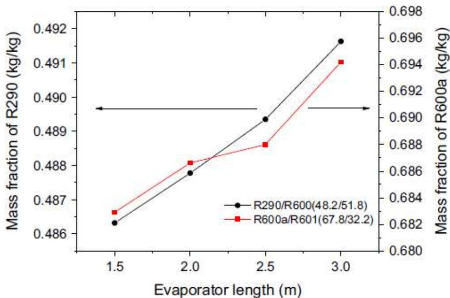
Fig 2.7 Evaporator length vs Mass fraction of R290/R600, R600a/R601 <sup>[9]</sup>
