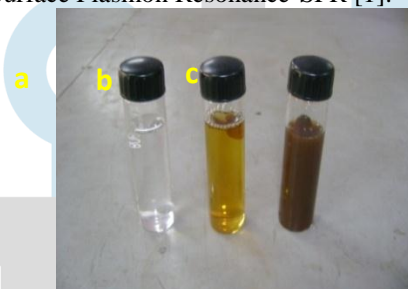
Fig 1. Optical photograph of (a) 1 mM AgNO 3 solution (b) Leaf extract (c) Leaf extract + AgNO 3 after 48 h of reaction
