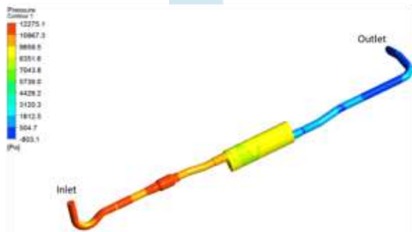
Case-2 Same system and exhaust tail pipe changed - \varnothing 93
