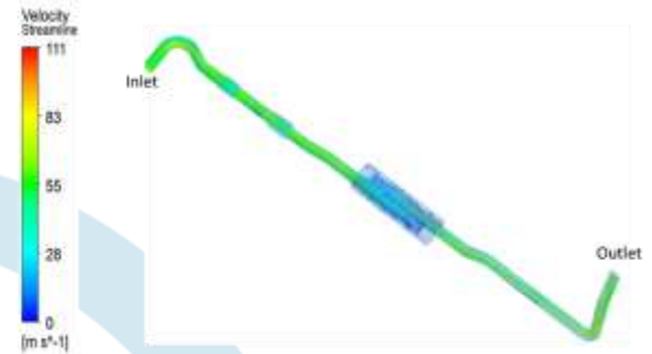
Case-1 Exhaust pipes \varnothing 101.6 mm.
