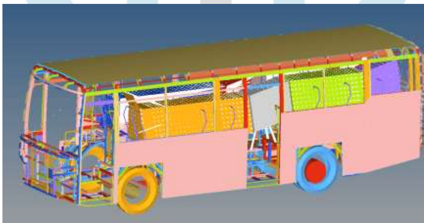
Figure 1: FE Model of complete bus structure
