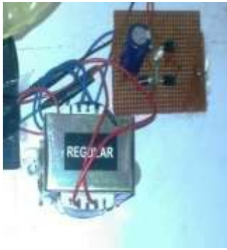
Fig.2. DC Power Supply
