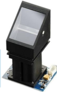
Fig. 2. Fingerprint Sensor (R305 - TTL)
