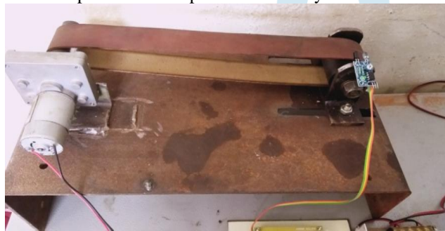
Fig No.9 Load conveyer setup
