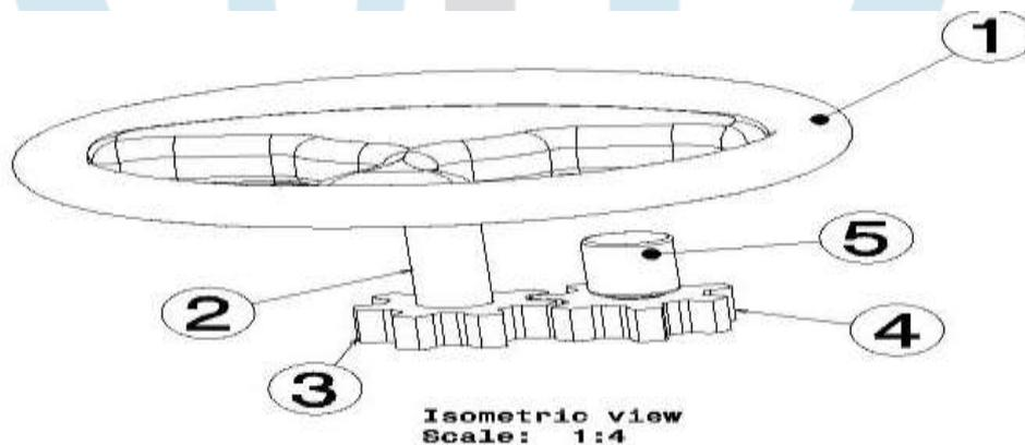
FIGURE 3: STEERING SYSTEM ASSEMBLY WITH ENCODER
