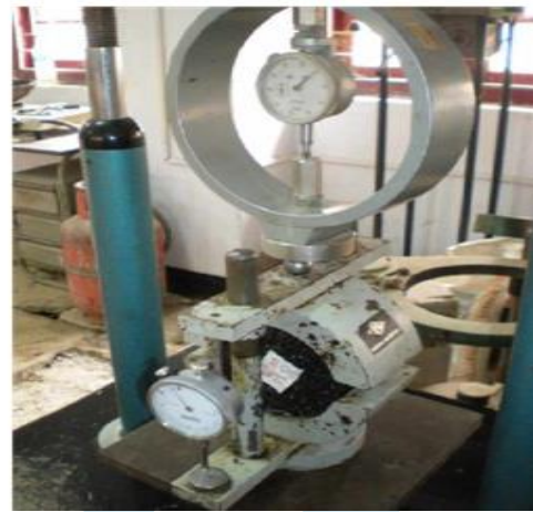
Fig 2 Marshall Test In Progress
