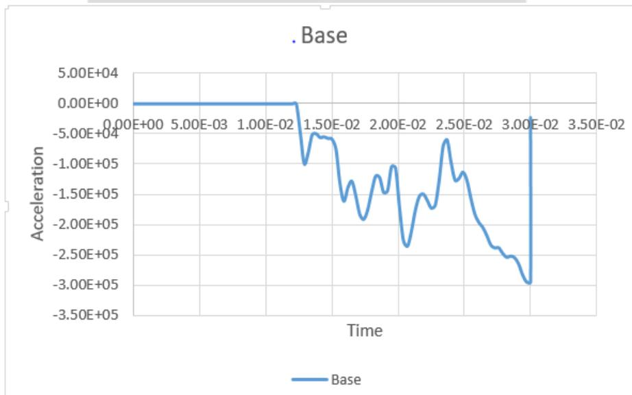
It was observed that the peak of acceleration was very high, so to control the peak value iteration were made. From the simulation it was necessary to increase the axial crushing and pure bending. Overall increasing the energy absorption and increasing the crash-worthiness of the vehicle.
