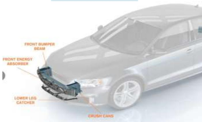
Figure 1: Bumper system of a car
