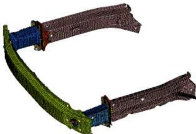
Figure 3: FEA Model of bumper system
