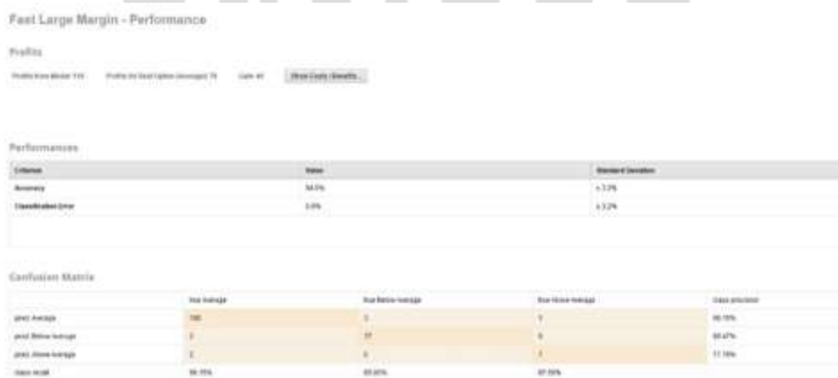
Figure 8: Error rate in this model was of 6.0%, with a class precision of 96.15% for Above Average, 89.47% for Average and 77.78% for Below Average
