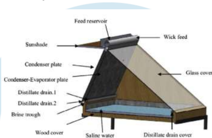
Figure: Design Parameters of Solar Still
