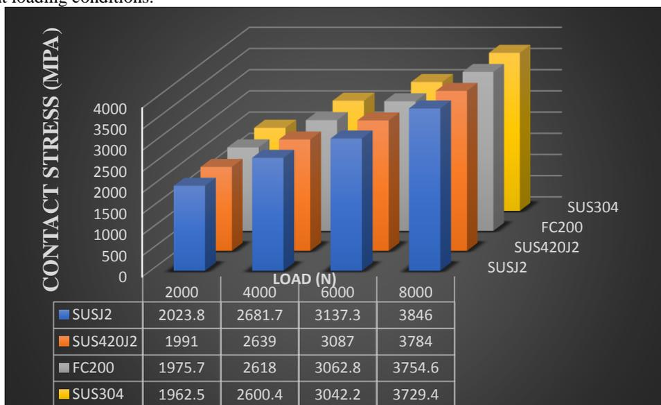
Fig.10 Shows the comparison of value of contact stresses in between ball and inner race
