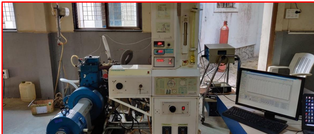
Fig 1: Shows the experimental setup of single cylinder four stroke diesel engine
