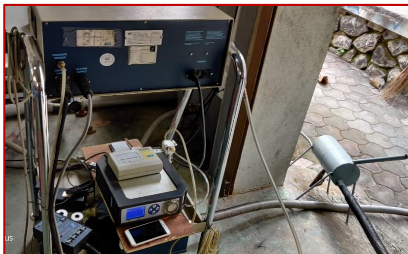
Fig 2: Shows Number: Psp 18, For Emission Testing Equipment used for measuring the exhaust gases
