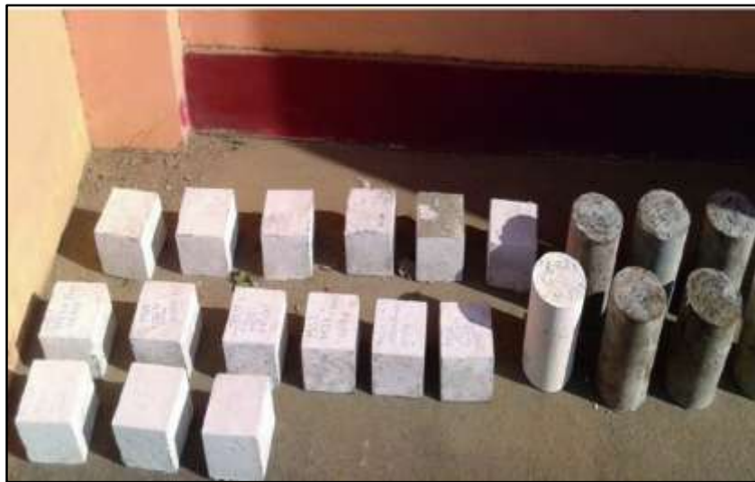
Figure 2:- Curing of modified GPC block.
