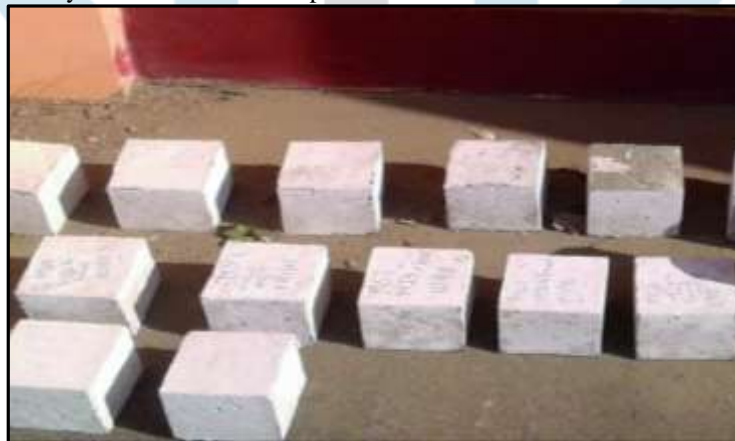
Figure 1:- Cubic block form of geopolymer concrete.
