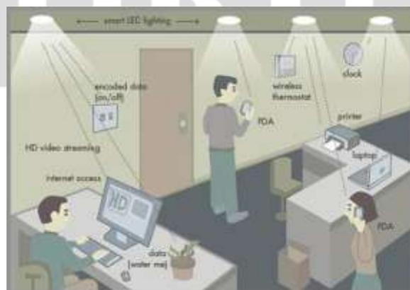
Fig 7: Li-Fi system connecting devices in a room (Source:[http://ijarjie.com/AdminUploadPdf/Review\\_Paper\\_on\\_Li\\_Fi\\_Light\\_Fidelity\\_ijarjie2056.pdf](http://ijarjie.com/AdminUploadPdf/Review_Paper_on_Li_Fi_Light_Fidelity_ijarjie2056.pdf))
