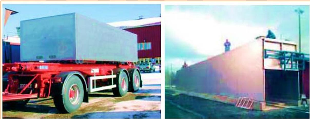
Figure 3. In the special container for gravel truck the stainless-steel sandwich panels as side walls are welded to wear resistant plates in the bottom of the structure.
