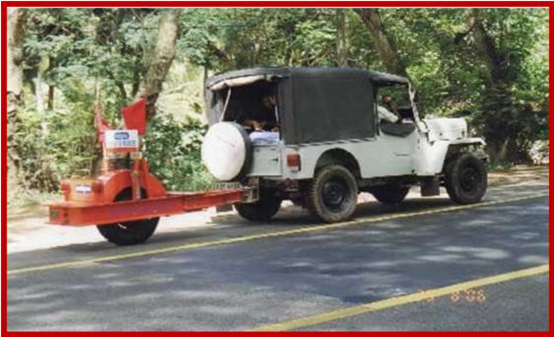
Fig: Roughness Survey in Progress
