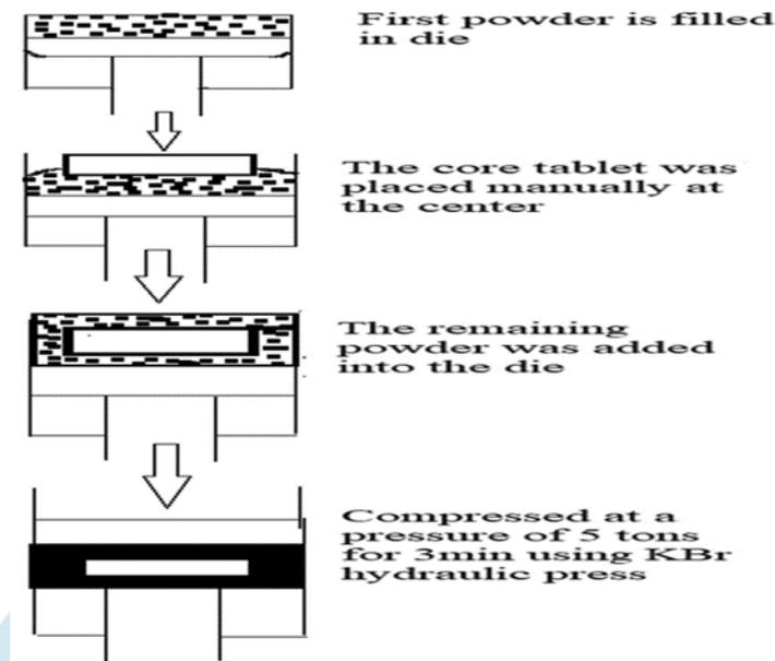
Figure. No. 08: press-coating technique
