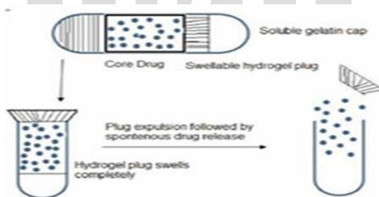
Fig.3: Design of Pulsincap system
