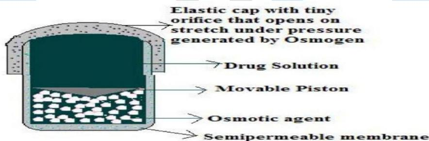
Figure. No. 05: System based on expandable orifice
