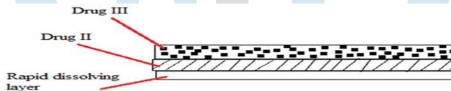
Figure. No. 09: Multilayered Tablet
