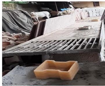
(fig4 compaction through a vibrating table)
