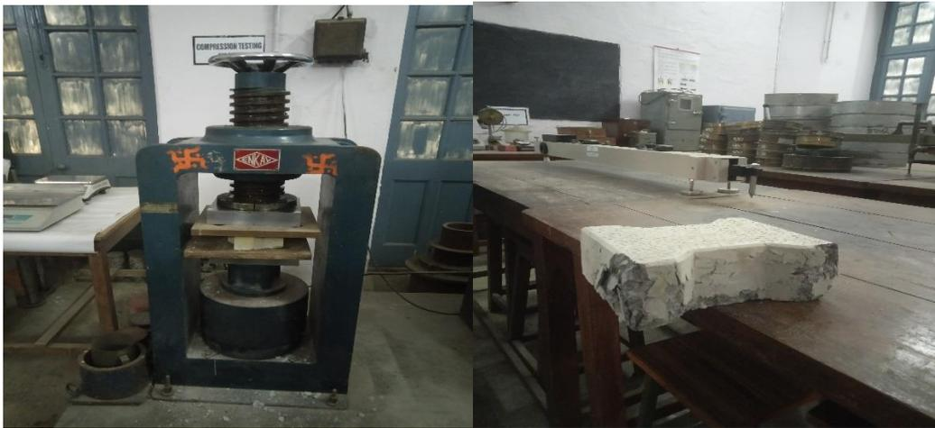
For loading, a CTM of 2000 kN was used [9]. Three samples have been evaluated in each category, and the formulation indicates the average compression value calculated by equation (1)
