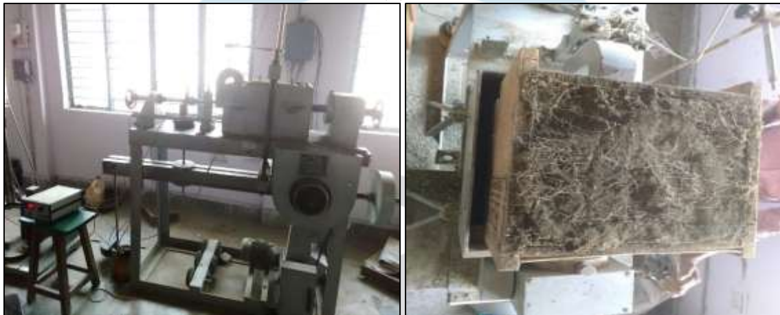
Fig. 9 Performing Large Shear Box Test on soil samples prepared with varying plant density
