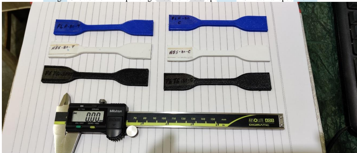
Fig.2 Shows the triangular and concentric set of samples for tensile testing
