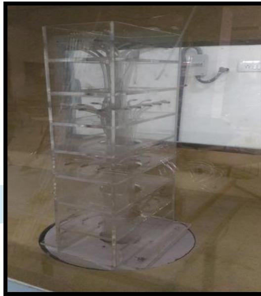
**Fig.2.4.2:** Solid (Acrylic) Model with pressure tapings
