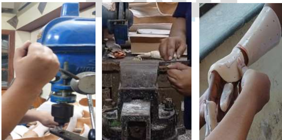
Fig. Drilling Machine, Shaping the component, LTTP Components molding on Subject
