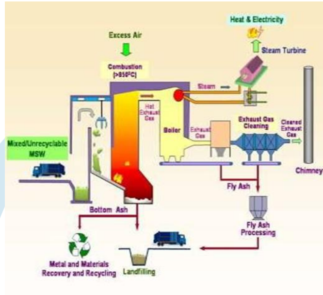
Fig. Process of incineration of MSW
