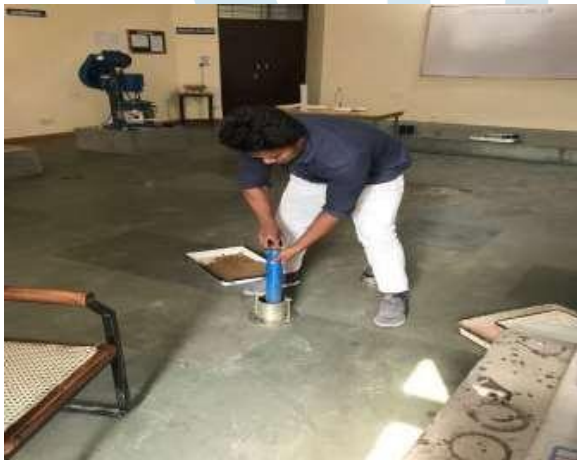
Fig. Test for CBR
