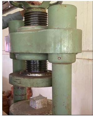
Fig – 10 : Compression testing
