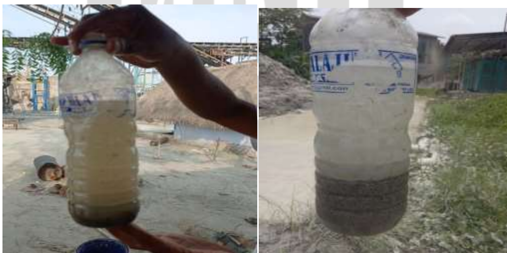
Fig No: 6 Slurry pH 12.5 Clarifier Over Flow : Cationic coagulant Polymer Application
