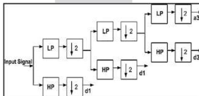
Figure 4 Block diagram of wavelet transform
