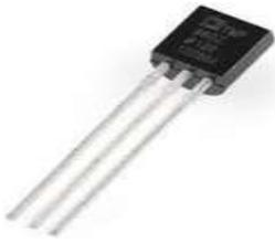
Figure 3. Temperature sensor
