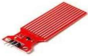
Figure 2. water level sensor
