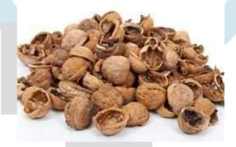
Walnut shells are a versatile abrasive media widely used in blasting, tumbling, cleaning, polishing, filtration, cosmetics, as well as non-skid applications and filler applications. Walnut shells are crushed, ground and classified to standard mesh sizes that range from coarse grio fine powders.
