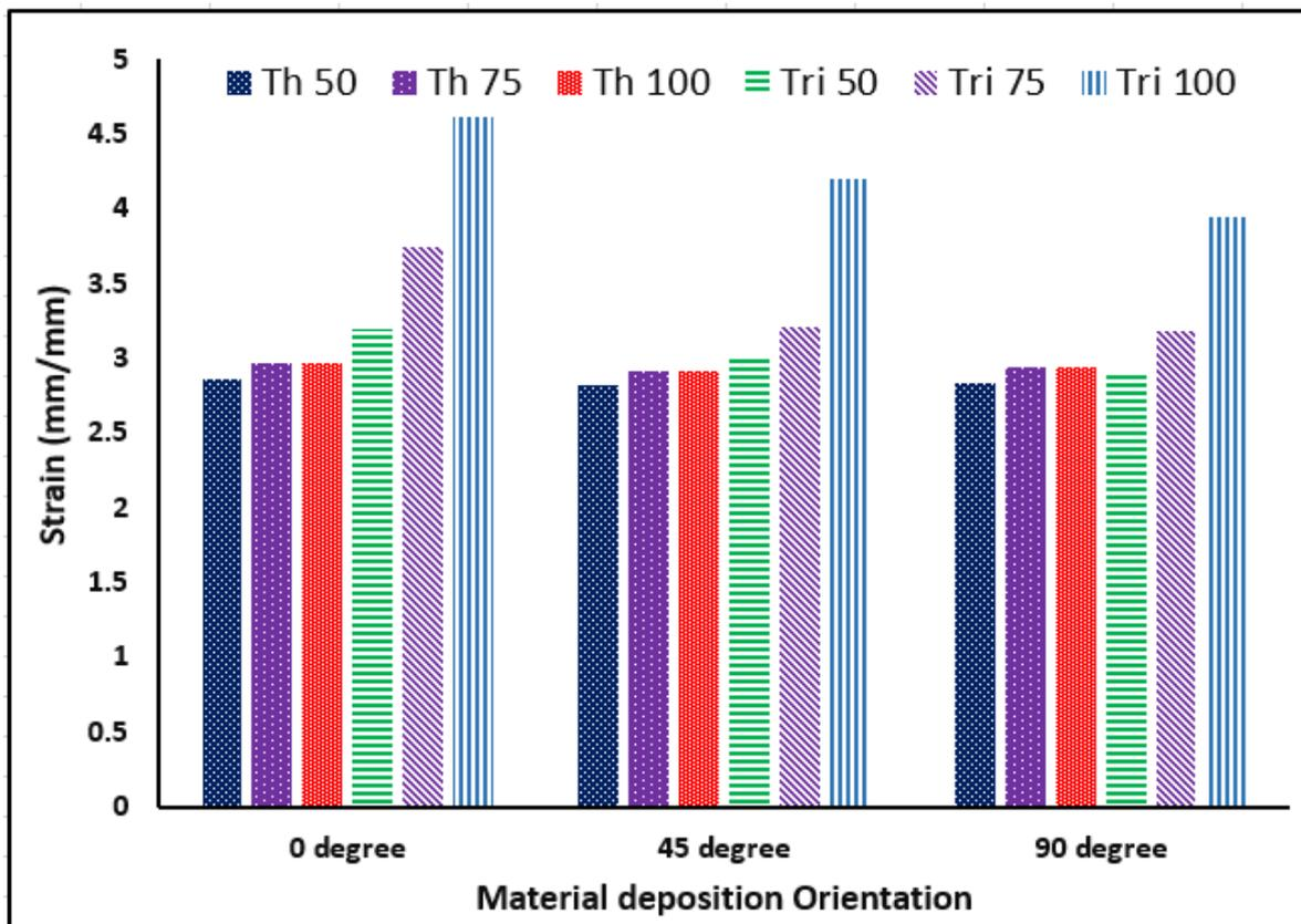
Fig 6. Comparison of strain at maximum tensile stress for a different set of experiments
