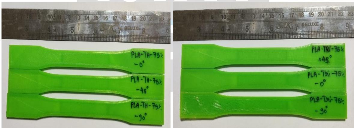
Fig 2. Tensile specimen having tri-hexagonal infill geometry with 75% infill density at different material deposition orientation
