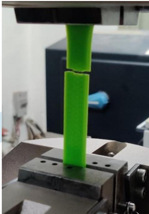
Fig 3. Tensile setup used for experimental testing of PLA specimen
