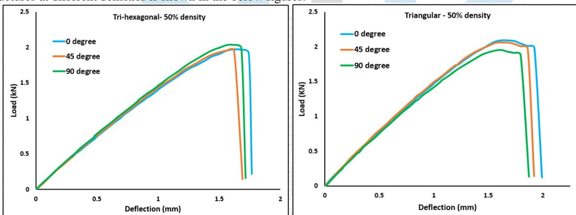
Fig 4. Load-deflection graph for 50% infill density with tri-hexagonal and triangular infill structure
