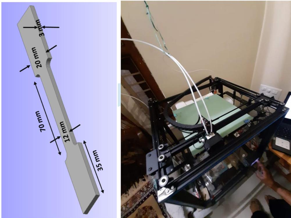
Fig 1. Shows the geometric specification of dog bone structure and printer used for 3D printing
