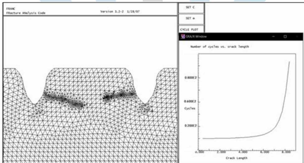
**Fig.8.** Quasi-static disc cutting modeling using the Paris criterion with FRANC2D
