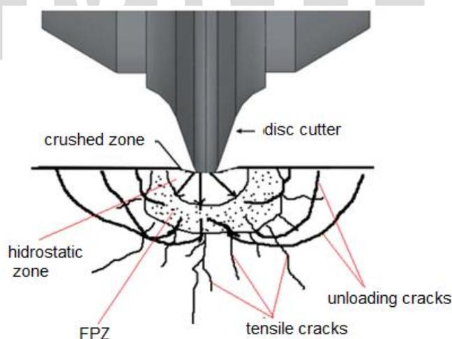
**Fig.10.** The crushed and cracked zones formed in the rock under the DCD
