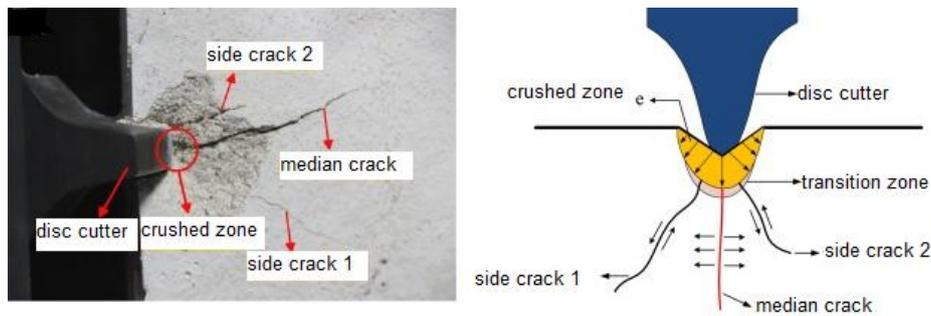
**Fig.2.** Crack and crushed zones under a disc cutter
