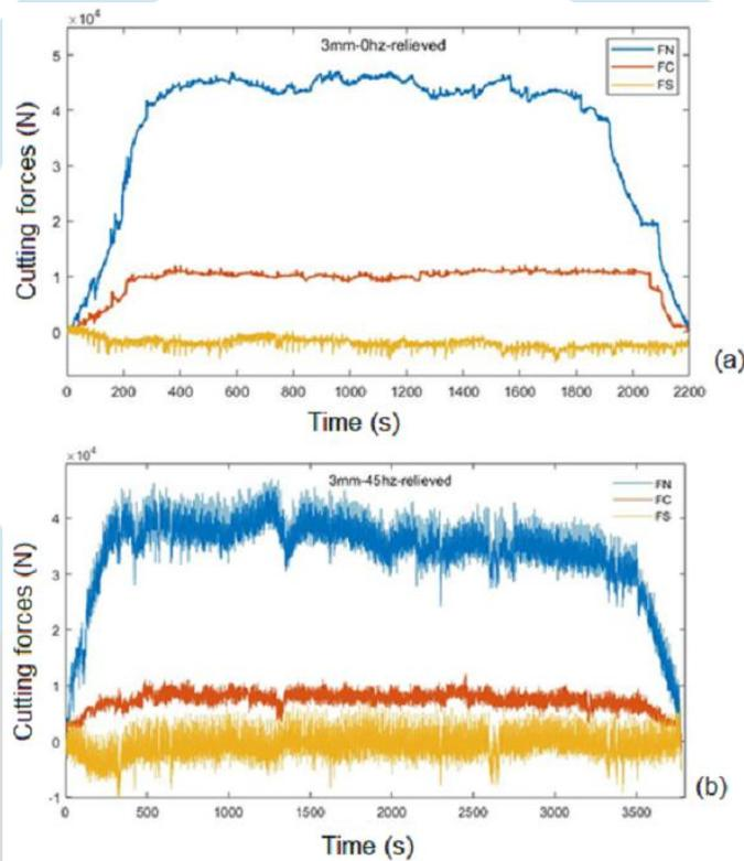
**Fig.6.** Comparison between (a) cutting forces of disc cutting without oscillation and (b) oscillating cutting with 45 Hz frequency
