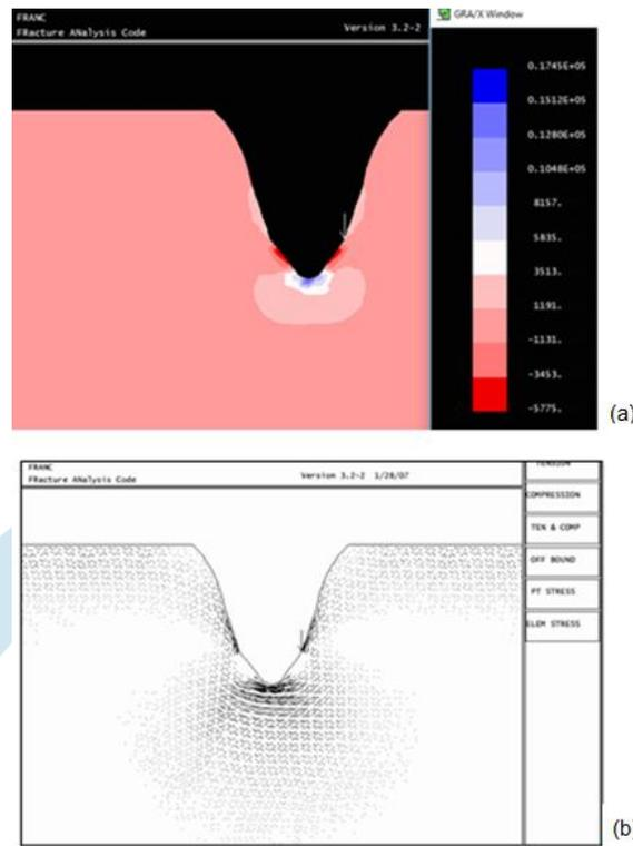
**Fig.7.** Stress distribution under a disc cutter (a) maximum principal stress (+) values are tensile and (-) values are compressive stresses (b) stress bar display of the tensile stress and concentration zones
