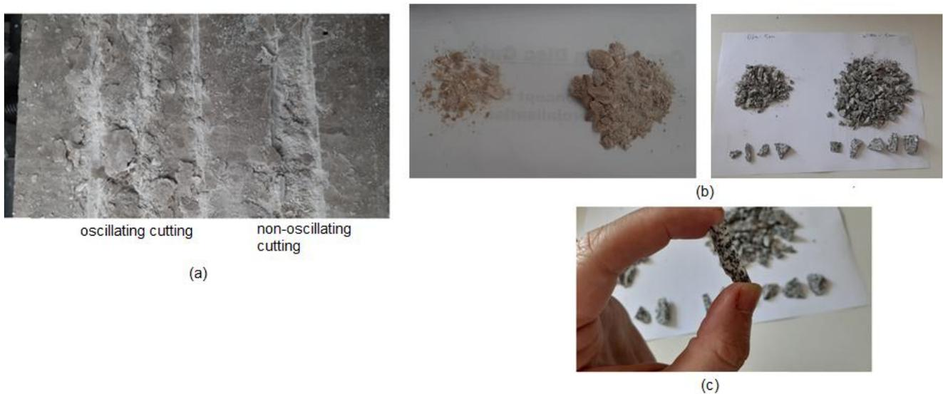
**Fig.9.** (a) Comparison between the cutting grooves obtained with the DCD and conventional disc cutter (b) cut and
