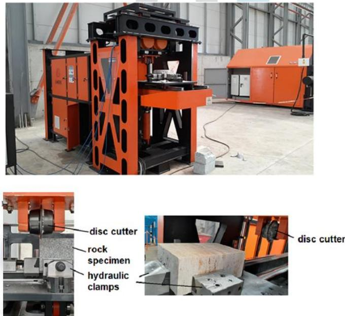
**Fig.3.** General view of the DCD technology prototype and a single oscillating disc cutter
