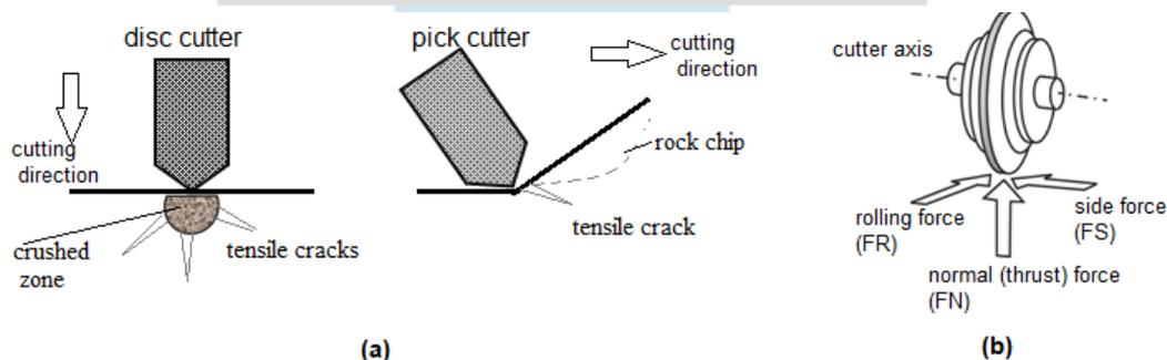
**Fig.1.** (a) Rock cutting directions of disc cutters and pick cutters, (b) cutting forces acting on a disc cutter
