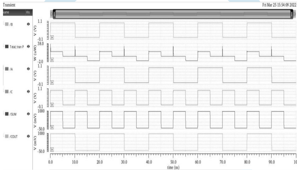
Fig 12: Simulation waveform for 1bit proposed GDI based Full adder
