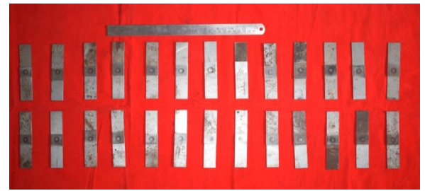
b) Specimen After Welding
