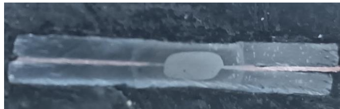
FIGURE 5.3 overview of macrostructure in welded DP-800 steel
