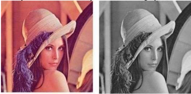
Figure 4.1 Converting from RGB to Grey
