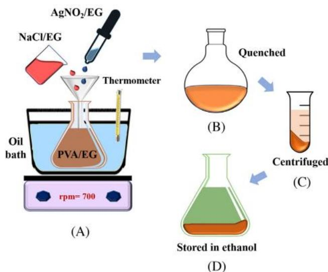
FIGURE 4 Steps to the synthesis of silver nanorods following polyol method: (A)  $\text{NaCl}/\text{EG}$  and  $\text{AgNO}_3/\text{EG}$  are added to  $\text{PVA}/\text{EG}$  solution and stirred at 700 rpm using magnetic stirrer, (B) quince at room temperature, (C) centrifuged at 6000 rpm, and (D) stored in ethanol by controlling the reaction temperature or nucleation process.[17]
