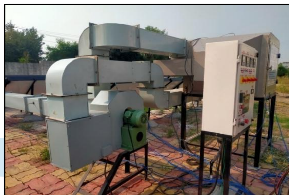
Fig.3: PV-thermal and packed bed collectors Fig.4: Ducting, drying chamber, control panel and blower
