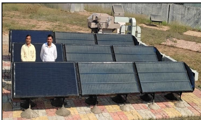
Fig.3: PV-thermal and packed bed collectors Fig.4: Ducting, drying chamber, control panel and blower
