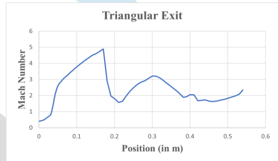
Figure 19 Triangular Jet Centreline Mach Variation
