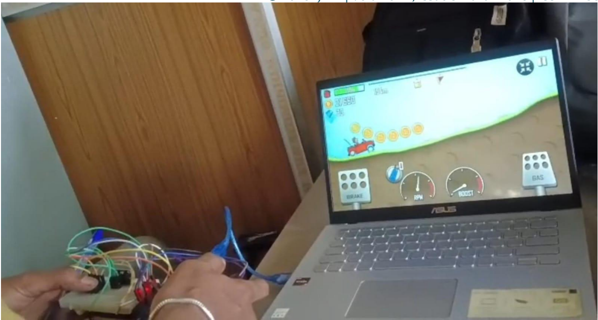
Figure 1: Physical prototype of the motion controller showing Arduino Uno, MPU6050 sensor, joystick and push buttons
