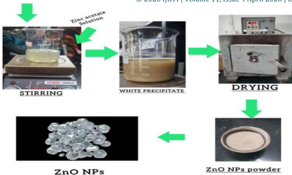
Fig-3: Schematic presentation: Preparation of Zinc Oxide Nanoparticles from Argemone mexicana Leaf Extract
