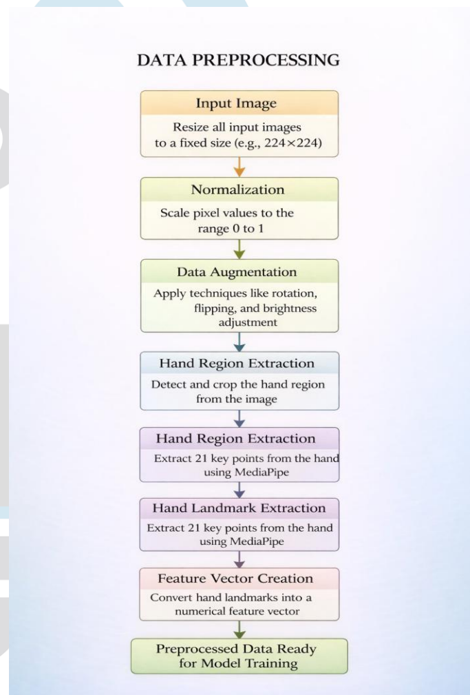
Fig. 3. Data preprocessing pipeline illustrating the transformation of input images into structured feature representations for effective model training.
