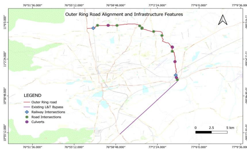
Fig 13. Outer Ring road Alignment and Infrastructure features
