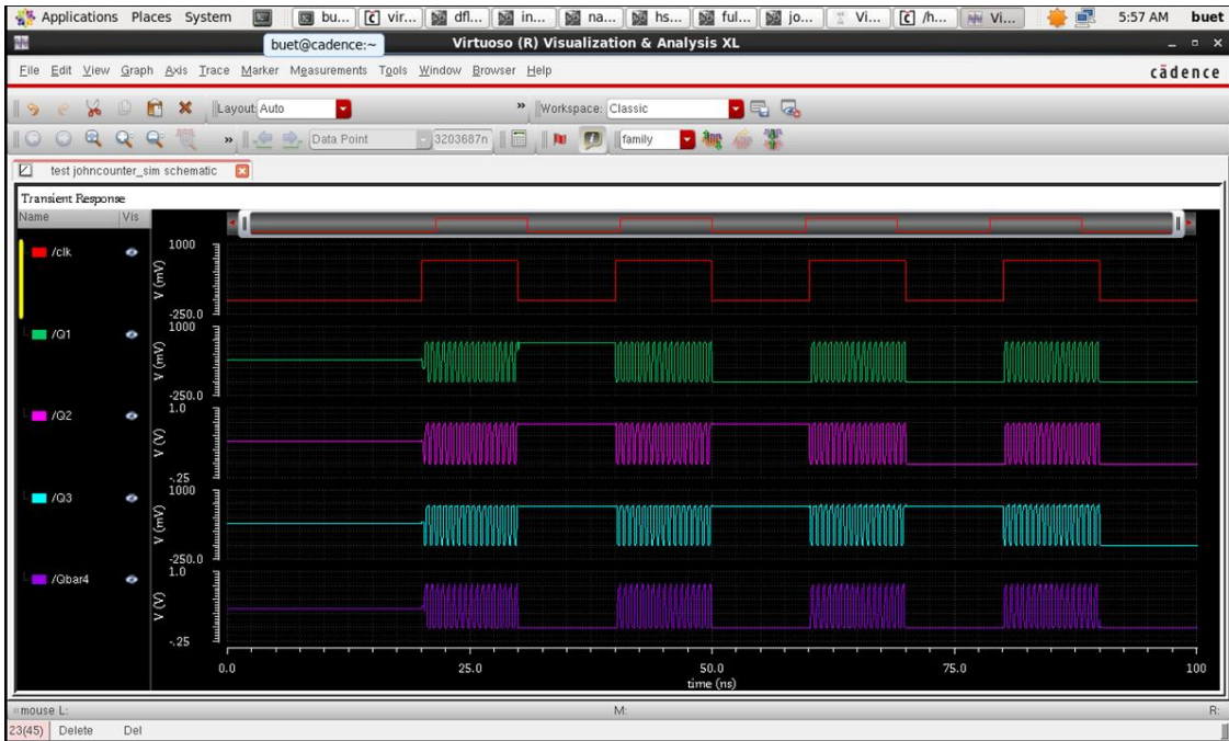
Fig. 8. Transient Response of Johnson Counter
