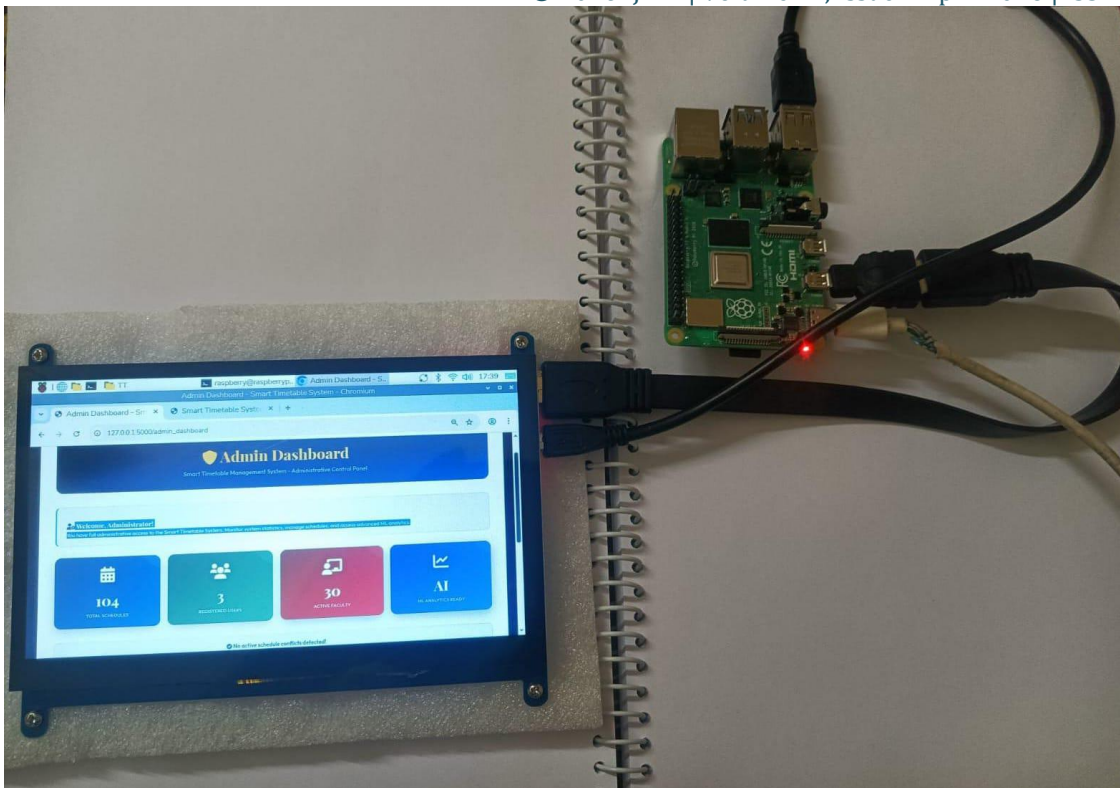
Fig. 7. Raspberry Pi 4 displaying the Admin Dashboard on a 7-inch LCD Display.
