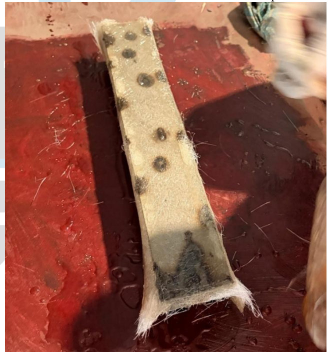
Fig - 28 Glass Fiber Reinforced Beam
